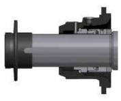
with quench, back to back double acting mechanical seal back to back or tandem, and double mechanical seals in tandem, Gland packing with or without flush and flushed packing seal.
