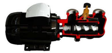
• RF Series: this is based on the same technology as the R Series, but in contrast uses support bearings with a plug-in shaft at the inlet. The RF Series can be directly connected to the drive via a flange. The ideal solution to supply as a bare shaft pump, while still maintaining a compact size and easy installation. The bearings ensure maximum reliability in all operating conditions.
