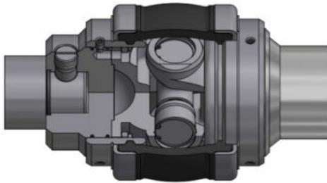
**Shaft sealing:** Different sealing systems can be installed, each solution being suitable to specific usage. The types available are: single mechanical seal, internal or external, single mechanical seal with quench, double mechanical seal back to back or tandem, gland packing with flush or without.
