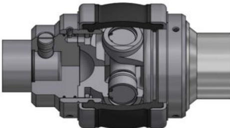
**Shaft sealing:** Different sealing systems can be installed, each solution being suitable to specific usage. The types available are: single acting mechanical seal, with quench, double acting mechanical seal back to back or tandem, Gland packing with or without flush.
