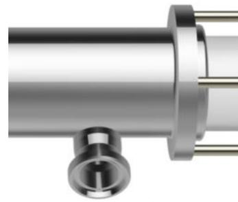
CIP connection built into pump body. This option enables insertion of washing fluid in the pump body to clean hygienic pumps in the best way possible. Manufactured tangential to the body, it avoids stagnation and enables efficient drainage of the fluids.
