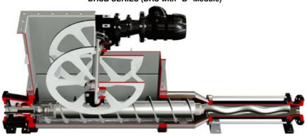
This model features a rectangular hopper and an enlarged auger feed screw that moves the product to the hydraulic part. The hopper is fitted with a "B" Module which features a special wheel device that feeds the screw to prevent bridging and increase flow ability of the plastic or pseudo plastic materials. Suitable for pumping non-flowing materials with up to 40% solids content with blocks that tend to bridging.
