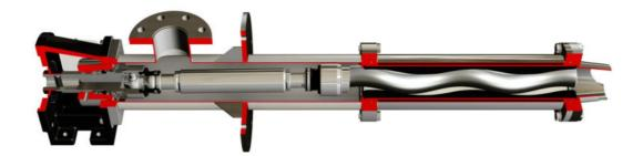
• **DV Long version:** This version requires to be fixed with a downhole support with the guiding cone to minimize the vibrations and oscillations of the pump caused by the considerable length of the pump itself.
