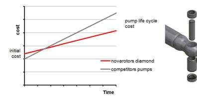
Maintenance: The Diamond series is designed to ensure easy maintenance and normally require the replacement of a minimum number of components. In particular the joint bushes are able to be replaced without having to replace shafts and rotors. The costs of maintenance are greatly reduced. The cost of the pump, considered in over its full life cycle, is highly competitive.
