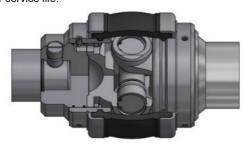
Joint protection: In the DHS or JHS series the joint rubber sleeve and clamp are protected from a particular device integrated inside the end of the auger feed screw. This characteristic is of considerable importance because it ensures the integrity of the joint in the case of pumping of abrasive substances or with solid blunt, without the needed to add expensive optional components.
