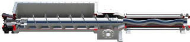
Model featuring a rectangular hopper, joint protection sleeves and enlarged auger feed screw to move the product to the hydraulic part designed for pumping silage in the Biogas sector. There are separate inlet features, a connection for the injection of liquids and a rectangular bottom for collecting any stones that might enter the hopper, with a large additional inspection hatch.
