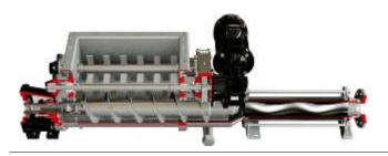
Model featuring a hopper with double bridge breaker shaft, joint protective sleeve and enlarged auger feed screw to move the product to the hydraulic part. Suitable for pumping highly viscous, non-flowing materials with up to 35% solids content prone to bridging or in blocks.
