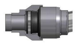
Coupling rod with auger feed screw. Improves transfer of dry, fibrous and non-sliding products in the body of the pump to improve the supply in the hydraulic part of the pump.
