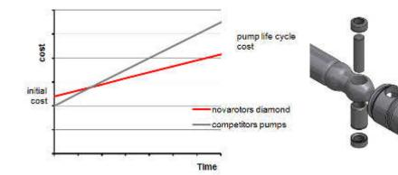
**Maintenance:** The Diamond series is designed to ensure easy maintenance and normally require the replacement of a minimum number of components. In particular the joint bushes allow the replace of the same without having to replace shafts and rotors. The costs of maintenance are really reduced. The cost of the pump, considered in his full life cycle, is highly competitive.
