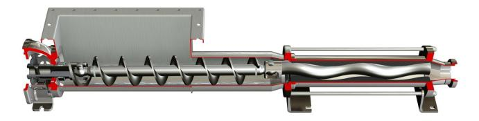
• **DHXC** serie: the DHXC series is a hygienic hopper pump with pin, standard to the DN series. This solution combines excellent sanitisation characteristics thanks to the design and casing completely free of dead zones and stagnation, together with the performance of the pin-type joint patented in the Diamond series. Lubrication of the pin is independent of the pumped product, therefore it is also suitable for abrasive fluids.
