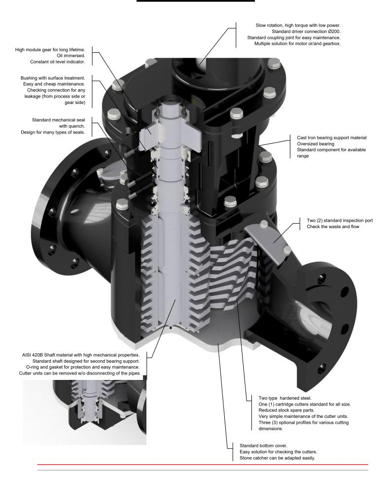
**Description 1**: Grinders installed on wastewater plant pipelines to reduce solids and protect pumps and filters.
