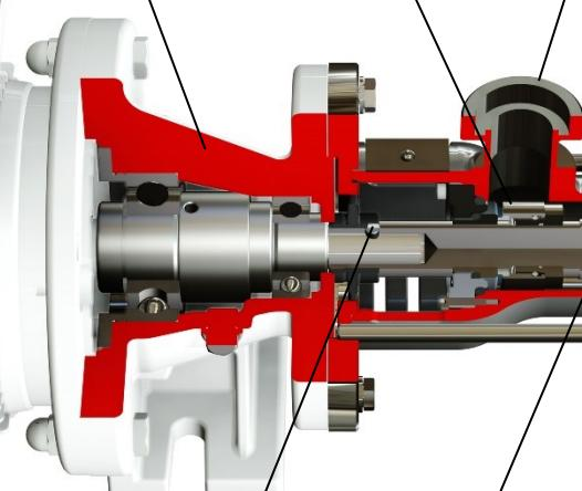
Ample suction sections enable excellent drying capacity and makes pumping of viscous substances efficient. Design free of dead zones or stagnation points. Polished casing for improved cleaning in CIP and SIP phases. Foodstuff fittings DIN 11851, DIN 11864 or Clamp ISO, ASME, DIN as standard
