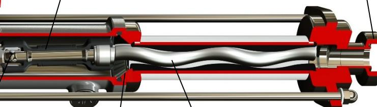
Connection via the pin to the drive or the bearing unit.
