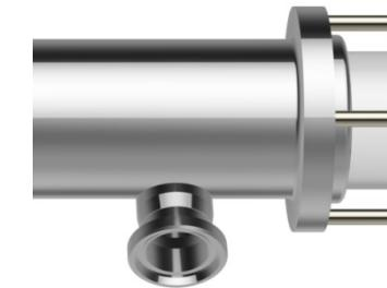
CIP connection built into pump body. This option enables insertion of washing fluid in the pump body to clean hygienic pumps in the best way possible. Manufactured tangential to the body, it avoids stagnation and enables efficient drainage of the fluids.
