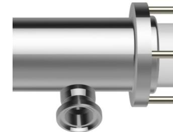
CIP connection built into pump body. This option enables insertion of washing fluid in the pump body to clean hygienic pumps in the best way possible. Manufactured tangential to the body, it avoids stagnation and enables efficient drainage of the fluids.
