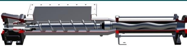
Standard model equipped with hopper and auger feed screw to move the product to the hydraulic part. Suitable for pumping materials with a low degree of flowability and prone to bridging.
