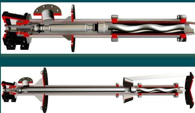
Vertical Series developed for pumping from tanks and wells immersed directly in the product to be pumped. The length can be adapted to suit the installation requirements. The stainless steel version (AISI 304 or AISI 316) is supplied with a stator jacket as standard to prevent corrosion of the stator. Two standard configurations are available: the short version and the long version with split casing and bottom mounted guiding cone.
