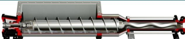
Model featuring a rectangular hopper, with joint protection sleeve and enlarged auger feed screw to move the product to the hydraulic part. Suitable for pumping high viscosity materials with low flowability and up to 28% solids content not prone to bridging.
