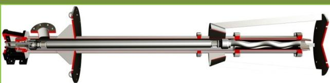
Vertical Series developed for pumping from tanks and wells immersed directly in the product to be pumped. The length can be adapted to suit the installation requirements. The stainless steel version (AISI 304 or AISI 316) is supplied with a stator jacket as standard to prevent corrosion of the stator. Two standard configurations are available: the short version and the long version with split casing and bottom mounted guiding cone.
