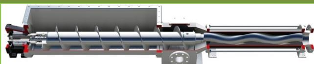
Model featuring a rectangular hopper, joint protection sleeves and enlarged auger feed screw to move the product to the hydraulic part designed for pumping silage in the Biogas sector. There are separate inlet features, a connection for the injection of liquids and a rectangular bottom for collecting any stones that might enter the hopper, with a large additional inspection hatch.
