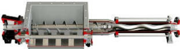
Model with enlarged hopper and auger feed screw to move the product to the hydraulic part, ideal for pumping materials with a low degree of flowability and prone to bridging. Standard AISI 304 or AISI 316 stainless steel construction.
